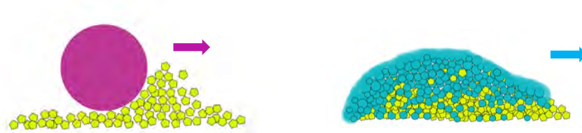
Figure 2: Normal fibers (left) versus microfibers (right) when used to pick up dirt and bacteria from a surface
