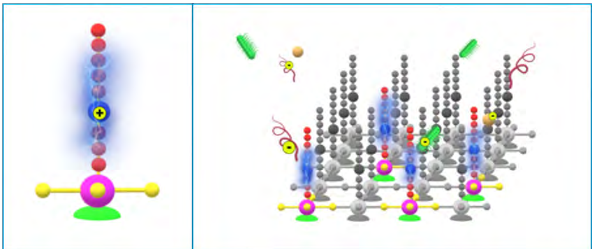
Figure 3: A visual representation of the mode of action of the antimicrobial treatment on the Supertowel. Pathogens are attracted by the positive charge on the carbon chains, and these then disrupt the cell wall, either physically or electrically, causing pathogens to be eliminated.
